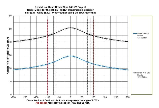
The audible noise at both the right and left right of way ("ROW") edge is 24.8 dB(A) (23.4 dB(A) at edge of ROW plus 25 feet) in fair weather and 46.3 dB(A) (44.9 dB(A) at edge of ROW plus 25 feet) in wet weather. The maximum noise that occurs within the ROW is 29.5 dB(A) in fair weather and 51 dB(A) in wet weather.
